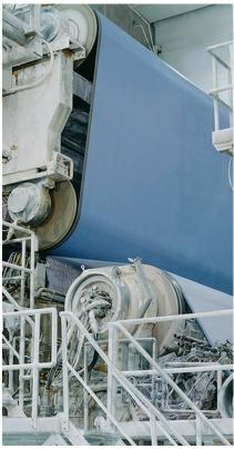
Paper lines have to operate without failures and problems, ideally round the clock 365 days a year. Paper webs that are 2,000 meters long and over 10 meters wide are produced from cellulose pulp or wastepaper within minutes, depending on the machine used.
